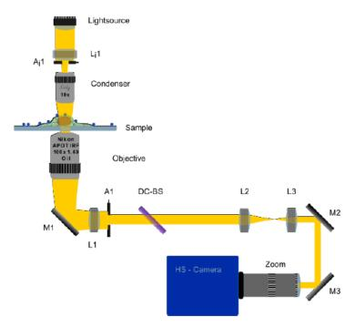
**Detection path schematic of the setup:** The sample is illuminated by a LED light-source operating in Koehler-illumination mode by lens *L*i1, Koehler-aperture Ai1 and the condenser. The image is formed by the objective and lens L1. It is further magnified by the lenses L2 and L3 before finally projected onto the CMOS chip of the high-speed camera by an adjustable zoom system.
